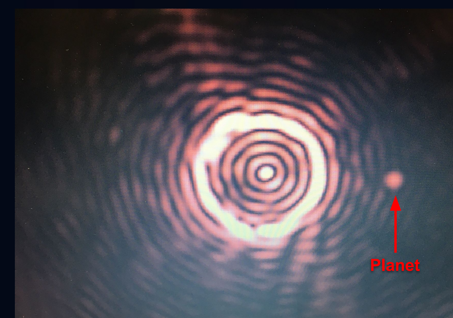
Fig. 6: Image with the FPM plus Lyot Stop; much of the starlight is suppressed and we can see objects around it clearer, like the simulated planet to the right.
